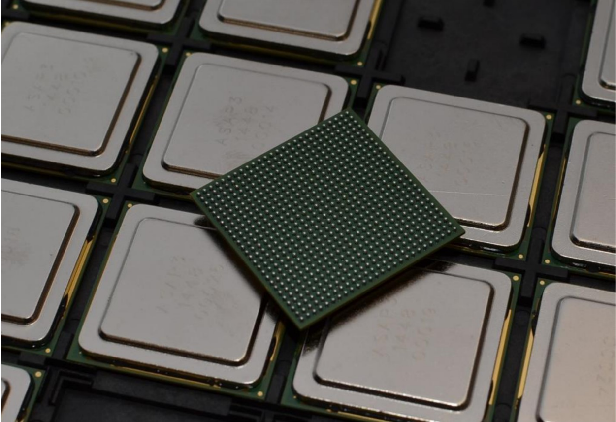
Figure 5.6: Underside of packaged KiloCore BGA package along with tray of packaged chips. The solder balls shown connect to the custom PCB daughtercard [8].
