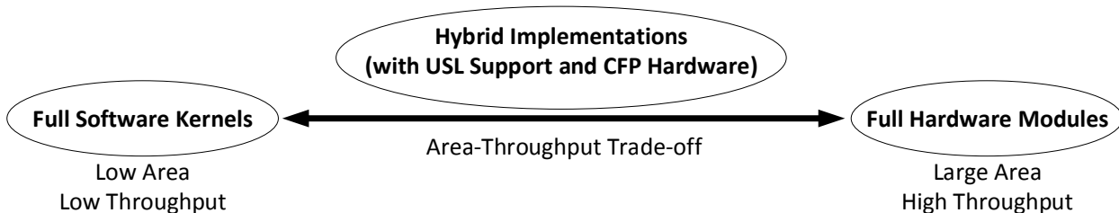
Figure 1.1: Hybrid implementations offer alternatives to pure-software and pure-hardware designs and enable a spectrum of designs with varying levels of chip area and throughput.
