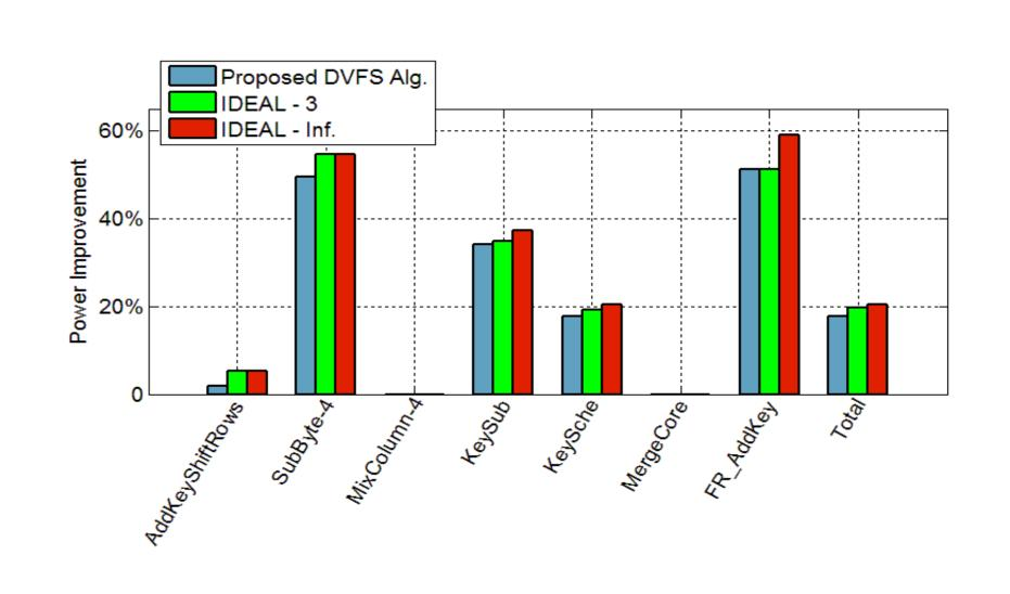
Proposed DVFS algorithm saves 18% power, which is only 3% less than theoretical limits
